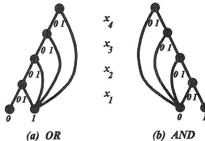
FIGURE 1. BDD's of the OR and AND Function on Four Variables
